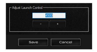
It is important to note that using Launch Control (also referred to as Anti-Lag) causes fuel to burn in the exhaust manifold and spin up the turbo. This means combustion will be happening in the manifold, turbo, and exhaust rather than just in the cylinders. More energy in the form of heat will be going into these exhaust components than normal and they will get hot quickly. Remember that the motor is water cooled, the exhaust manifold is not!
