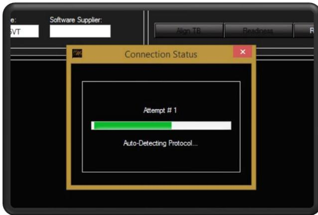
Connect establishes a direct connection between the Windows device and the vehicle's ECU. Clicking "**Connect**" launches the connection dialog which gives a brief description of the connection status while making a maximum of 5 attempts to connect with a supported ECU.
