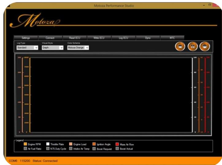
For an initial data log, it is recommended to allow 20 min for the vehicle to adapt before logging any data. A log should be performed to make sure things are running as expected. The best way to log initially is mixed mode driving, providing a little bit of idle, part throttle, acceleration and deceleration about 15 mins of logging works well.
